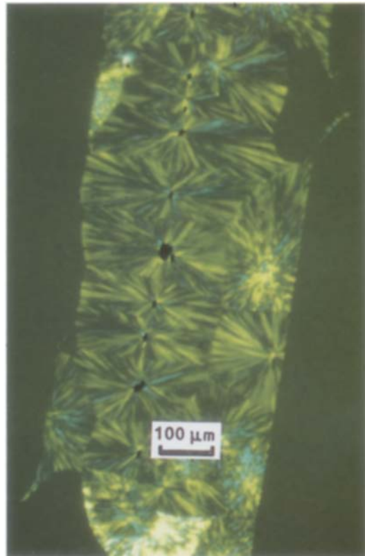
Figure 4 Cross-section of HM carbon fibres in polypropylene crystallized at 135°C.
